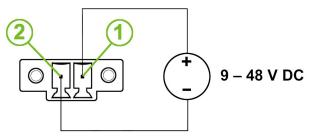
Figure 9: Connection of Power Supply
