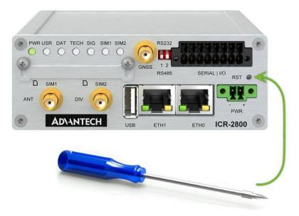
Figure 16: Resetting the Router
