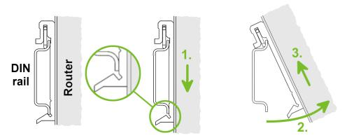
Figure 5: Removing Router from the DIN Rail
