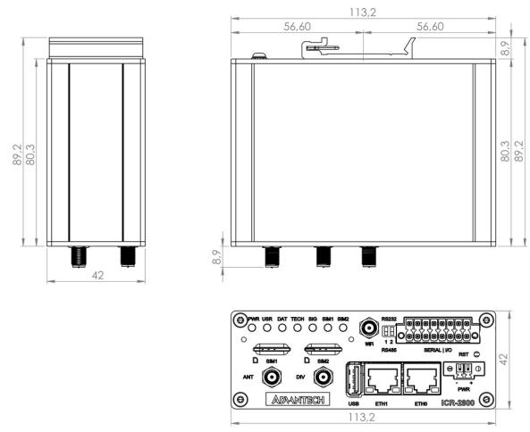
Figure 2: Metal Box - Top, Side and Front View
