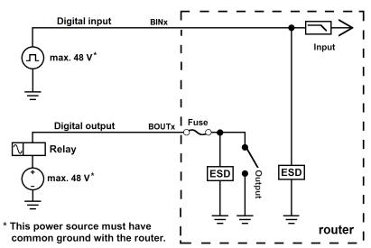
Figure 12: Functional Scheme of the Binary Interface
