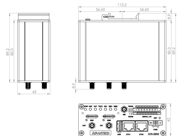
Figure 2: Metal Box - Top, Side and Front View
