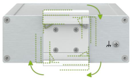
Figure 4: Position of the DIN Rail Clip
