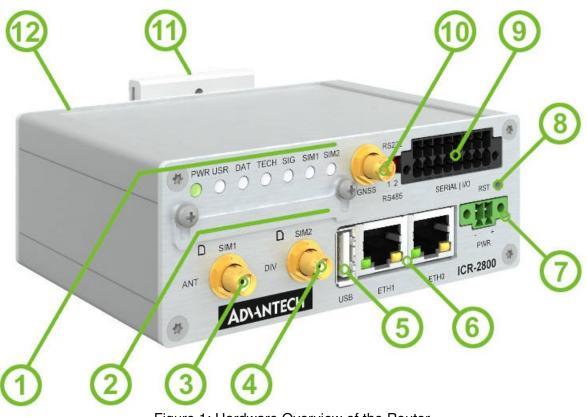
Figure 1: Hardware Overview of the Router
