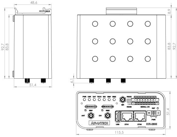
Figure 3: Plastic Box - Top, Side and Front View
