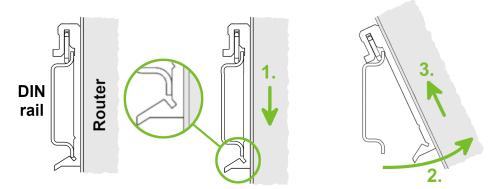
Figure 5: Removing Router from the DIN Rail
