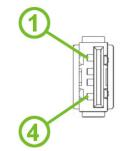
Figure 15: USB Connector Pinout
