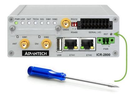
Figure 16: Resetting the Router
