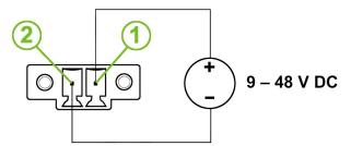
Figure 9: Connection of Power Supply
