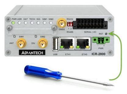
Figure 20: Resetting the Router
