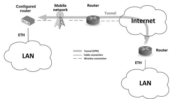
Figure 3: Using VPN Tunnel
