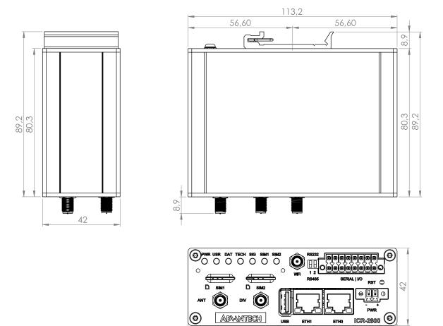
Figure 6: Metal Box – Top, Side and Front View
