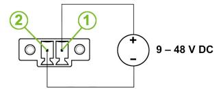
Figure 13: Connection of Power Supply
