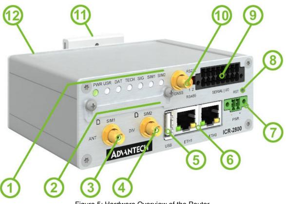
Figure 5: Hardware Overview of the Router
