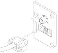
Figure 20: Connection of power supply connector
