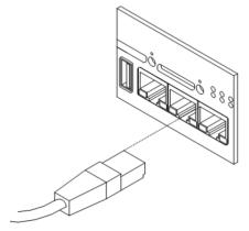
Figure 26: Connection of ethernet cable
