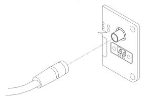
Figure 23: Connecting of the antenna
