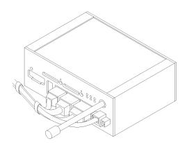
Figure 12: Cable routing for SL version
