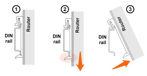
Figure 16: Removal from the DIN rail
