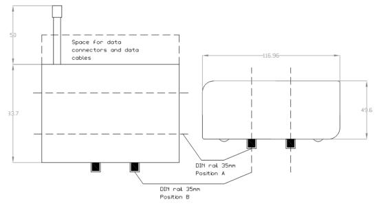
Figure 7: Basic dimensions of plastic box
