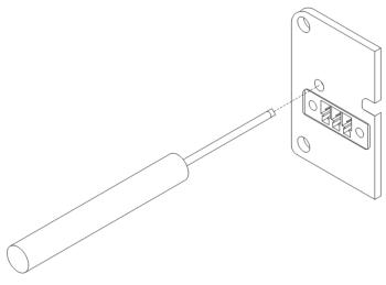
Figure 36: Router reset
