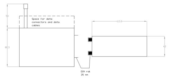
Figure 8: Basic dimensions of metal box
