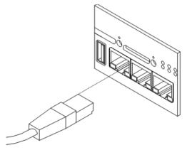
Figure 28: PORT1 cable connection
