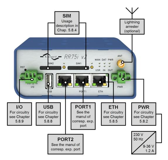
Figure 37: Router connection
