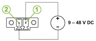
Figure 9: Connection of Power Supply
