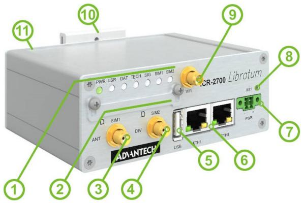
Figure 1: Hardware Overview of the Router
