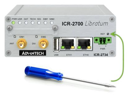
Figure 12: Resetting the Router
