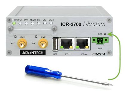
Figure 15: Resetting the Router
