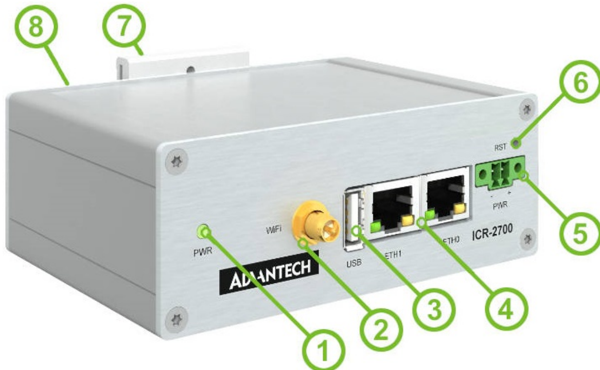
Figure 1: Hardware Overview of the Router
