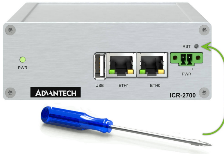
Figure 11: Resetting the Router
