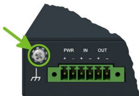
Figure 13: Grounding screw position
