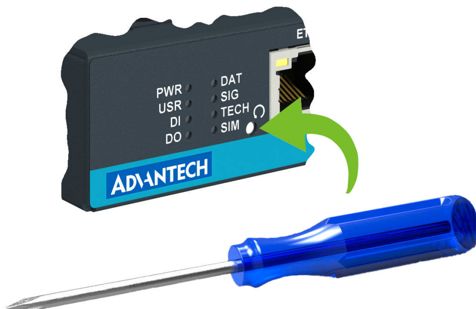
Figure 17: Resetting the router
