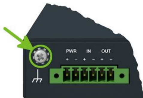
Figure 13: Grounding screw position
