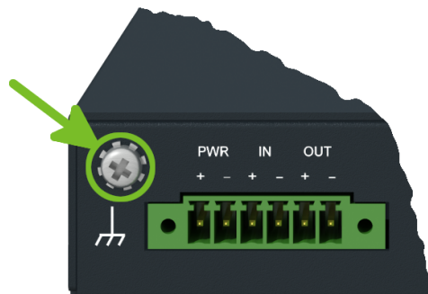
Figure 16: Position of the Grounding Screw
