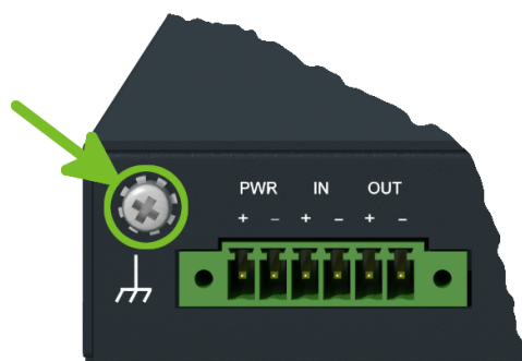
Figure 16: Position of the Grounding Screw
