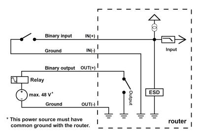
Figure 17: Functional Scheme of the Binary Interface
