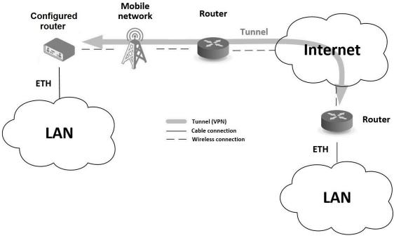
Figure 3: Using VPN Tunnel
