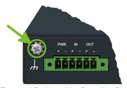
Figure 12: Position of the Grounding Screw
