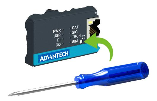
Figure 16: Resetting the Router
