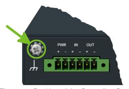
Figure 12: Position of the Grounding Screw
