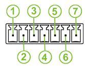
Figure 15: RS485 and RS232 Pinout
