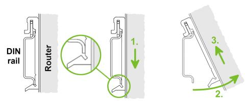
Figure 7: Removing Router from the DIN Rail
