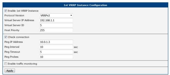
Figure 24: Example of VRRP Configuration - Main Router
