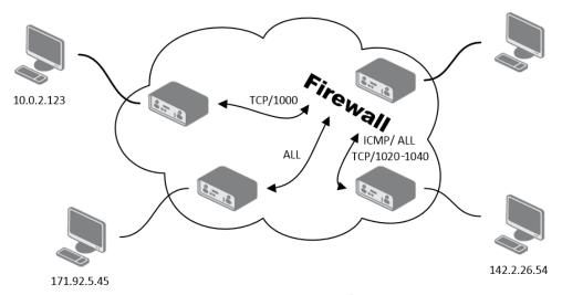
Figure 48: Topology for the IPv4 Firewall Configuration Example
