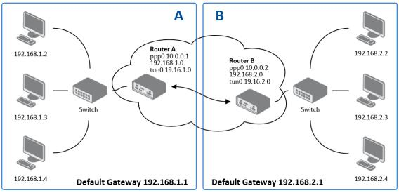
Figure 56: Topology of OpenVPN Configuration Example
