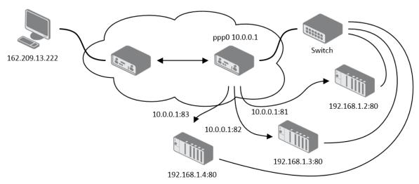
Figure 53: Topology for NAT Configuration Example 2
