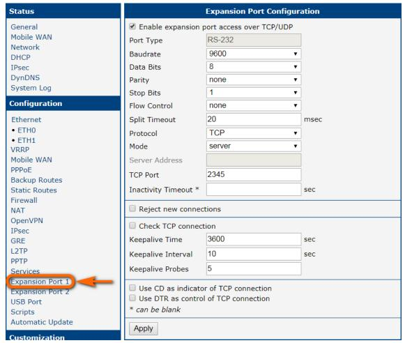
Figure 130: Serial Gateway – konfigurace Expansion Port 1
