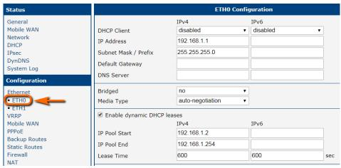
Figure 120: Access to the Internet from LAN – Ethernet configuration
