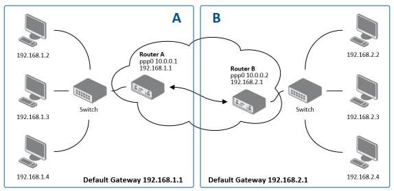
Figure 68: Topology of PPTP Tunnel Configuration Example
