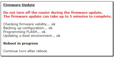
Figure 117: Process of Firmware Update
