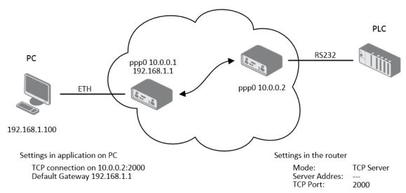
Figure 88: Example of Ethernet to serial communication configuration
