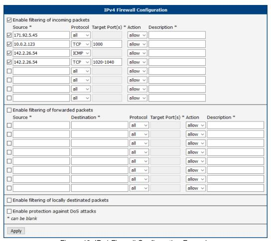
Figure 49: IPv4 Firewall Configuration Example
