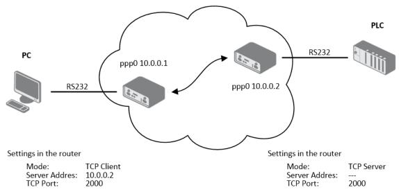
Figure 89: Example of serial interface configuration
