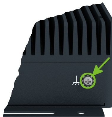
Figure 14: Position of the grounding screw
