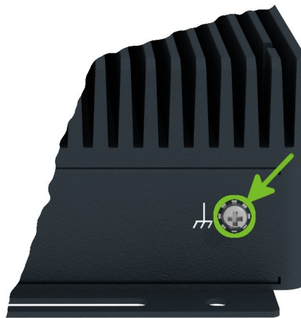
Figure 18: Position of the Grounding Screw
