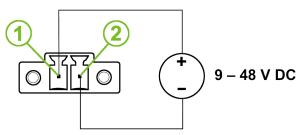
Figure 17: Power Connector Pinout
