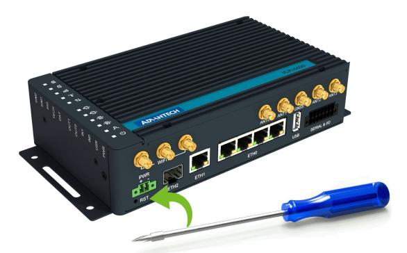
Figure 24: Resetting the Router
