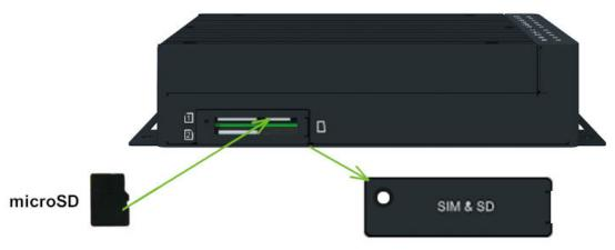
Figure 23: MicroSD Card Insertion
