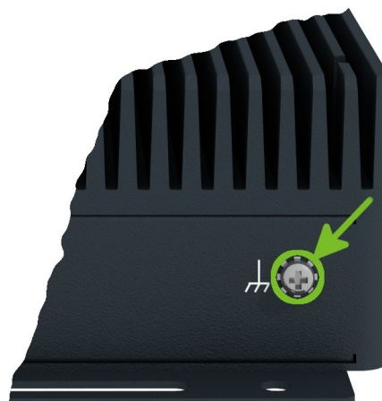
Figure 14: Position of the Grounding Screw
