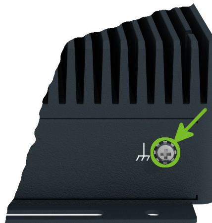
Figure 18: Position of the Grounding Screw
