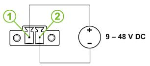
Figure 17: Power Connector Pinout
