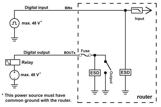
Figure 20: Functional Scheme of the Digital Interface
