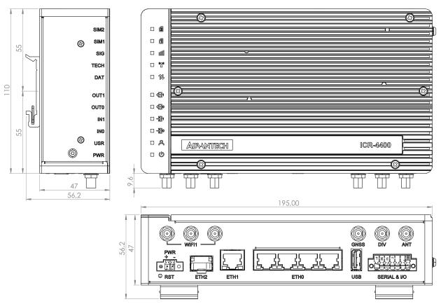
Figure 8: Router Dimensions - Front, Top and Right view with DIN holder
