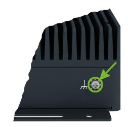
Figure 18: Position of the Grounding Screw
