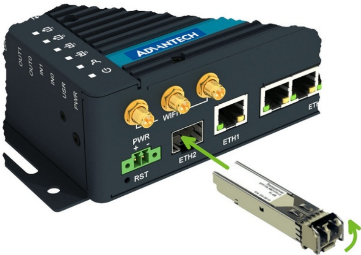
Figure 12: SFP module installation
