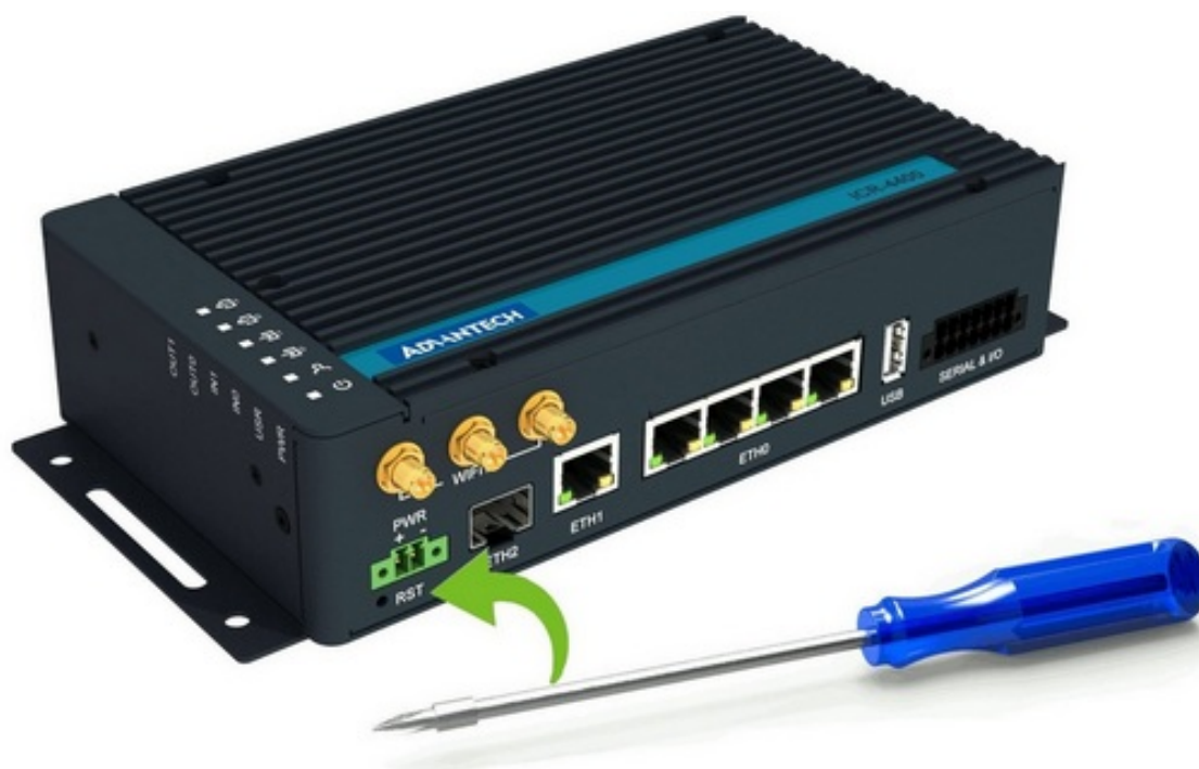
Figure 20: Resetting the router
