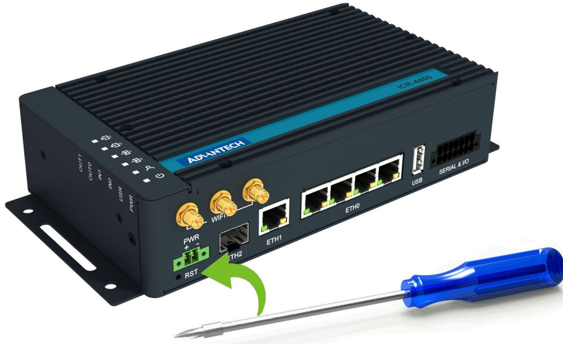
Figure 19: Resetting the Router
