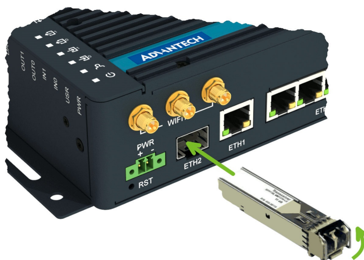
Figure 11: SFP Module Installation
