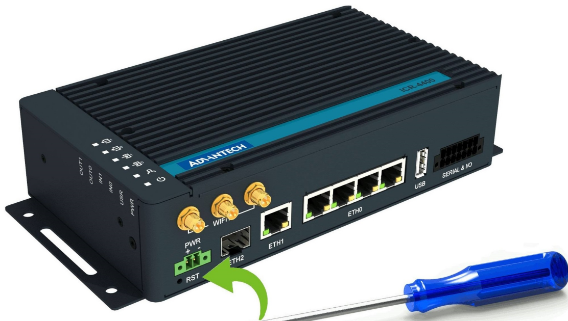
Figure 19: Resetting the Router
