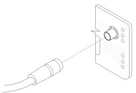
Figure 29: Connecting of the antenna
