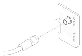
Figure 29: Connecting of the antenna
