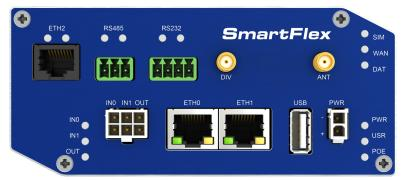
Figure 46: Version with RS232-RS485-ETH interface
