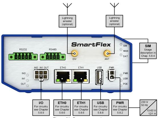
Figure 50: Router connection
