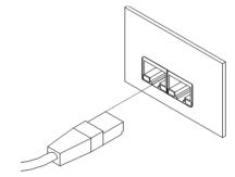
Figure 35: Connection of Ethernet cable
