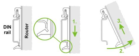
Figure 25: Removal from the DIN rail
