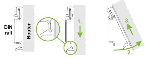
Figure 10: Removing Router from the DIN Rail
