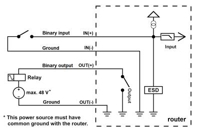
Figure 17: Functional Scheme of the Digital Interface
