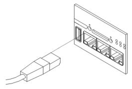
Figure 27: PORT2 cable connection
