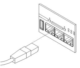
Figure 26: PORT1 cable connection
