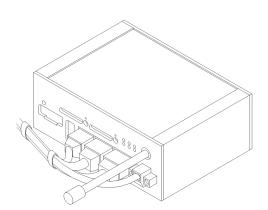
Figure 14: Cable routing (metal)
