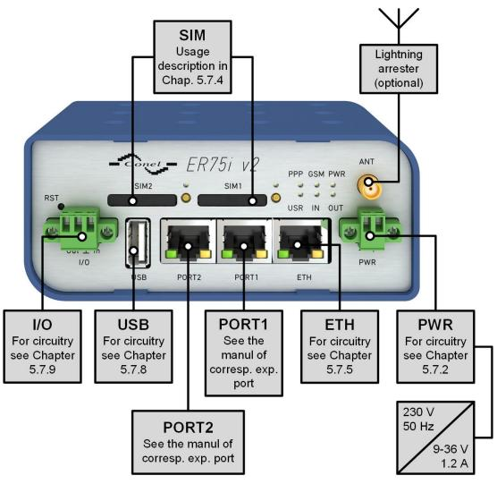
Figure 33: Router connection
