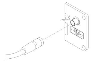
Figure 22: Connecting of the antenna
