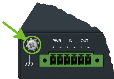
Figure 12: Position of the Grounding Screw
