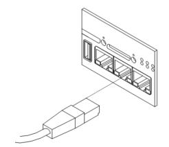
Figure 25: Connection of ethernet cable
