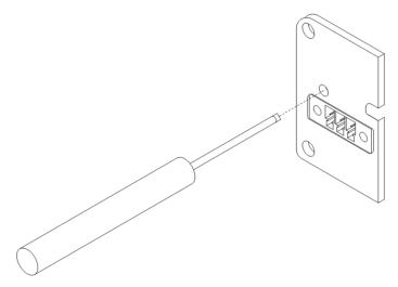
Figure 32: Router reset
