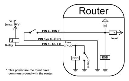
Figure 31: Connection of input and output to the router
