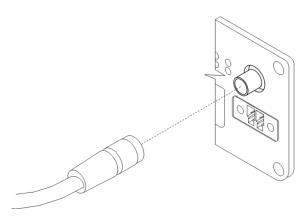
Figure 22: Connecting of the antenna
