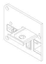
Figure 23: Ejected SIM holder
