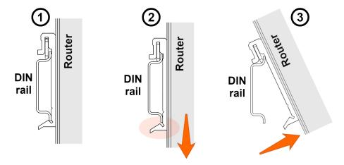
Figure 18: Removal from the DIN rail
