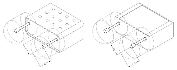
Figure 11: Space around antennas (plastic) Figure 12: Space around antennas (metal)
