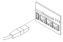
Figure 27: PORT2 cable connection
