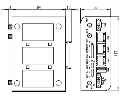
Figure 9: Basic dimensions of plastic box (bottom and front view)
