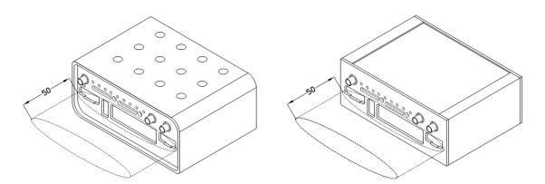
Figure 15: Space in front of connectors (plastic) Figure 16: Space in front of connectors (metal)
