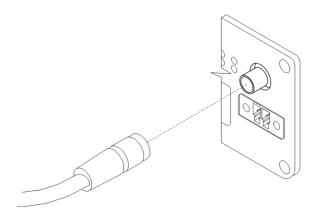
Figure 22: Connecting of the antenna
