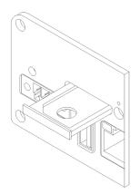
Figure 23: Ejected SIM holder
