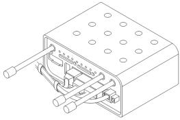
Figure 13: Cable routing (plastic)
