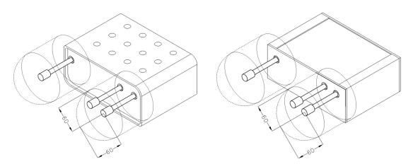
Figure 11: Space around antennas (plastic) Figure 12: Space around antennas (metal)
