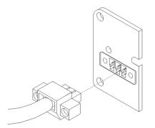
Figure 30: Connection of I/O cable
