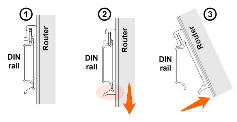
Figure 18: Removal from the DIN rail
