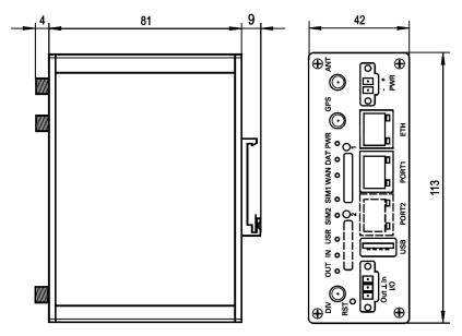
Figure 10: Basic dimensions of metal box (bottom and front view)
