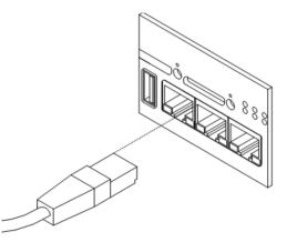
Figure 26: PORT1 cable connection
