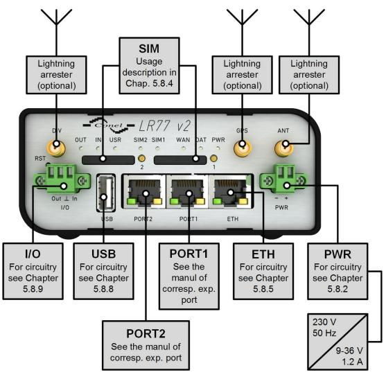
Figure 33: Router connection
