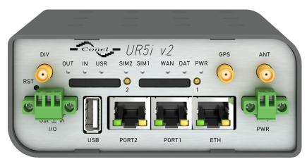
Figure 17: Front panel UR5i v2F
