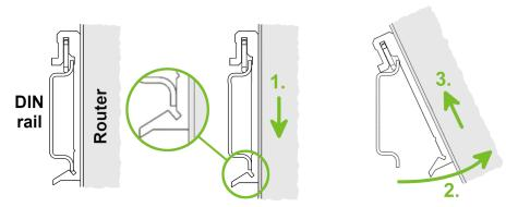
Figure 25: Removal from the DIN rail
