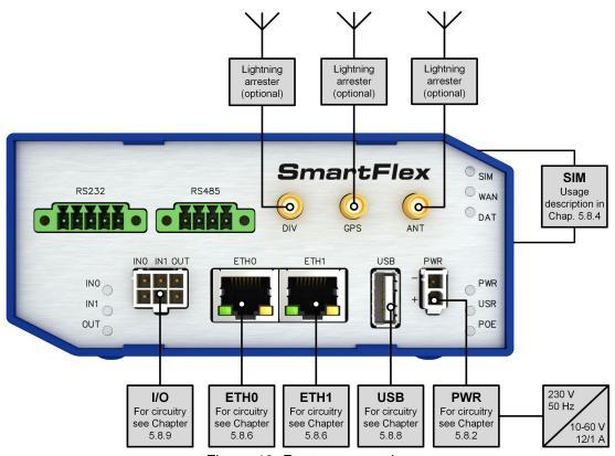
Figure 48: Router connection
