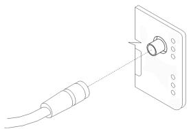
Figure 29: Connecting the antenna
