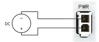
Figure 28: Connection of Power Supply
