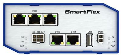
Figure 23: Version with SWITCH board
