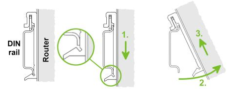
Figure 9: Removal from the DIN rail
