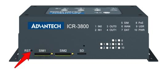
Figure 11: Router reset
