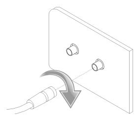
Figure 19: Connecting the antenna
