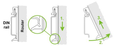
Figure 14: Removal from the DIN rail
