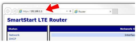
Figure 26: Entering the IP address of the router
