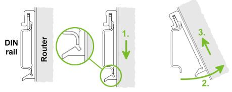
Figure 7: Removing from the DIN rail
