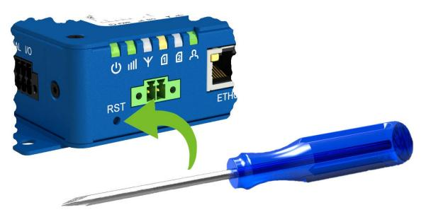
Figure 15: Resetting the Router
