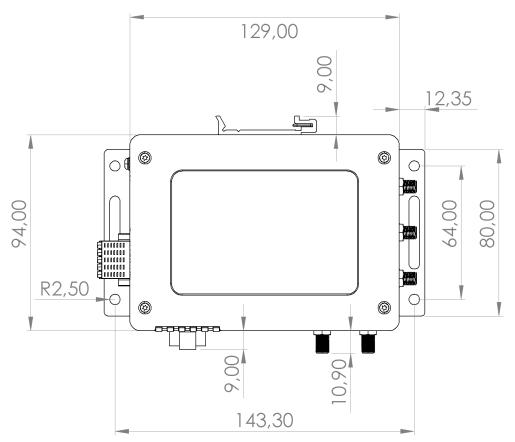
Figure 4: Basic dimensions of the router box
