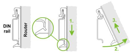
Figure 7: Removing from the DIN rail
