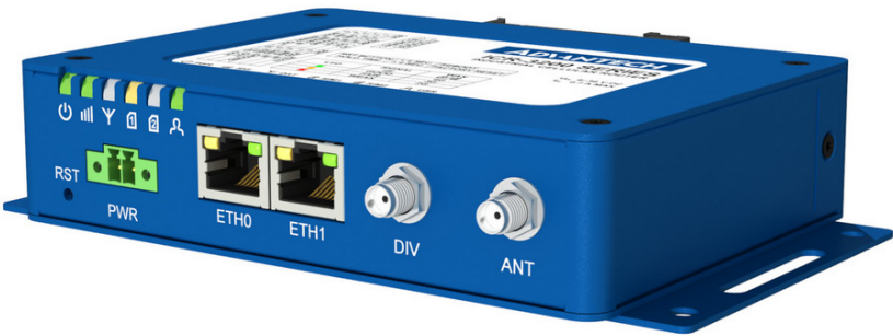
Figure 2: Version without WiFi and GNSS
