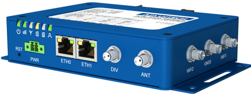
Figure 3: Version with WiFi and GNSS
