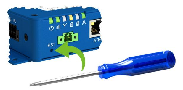
Figure 19: Resetting the Router
