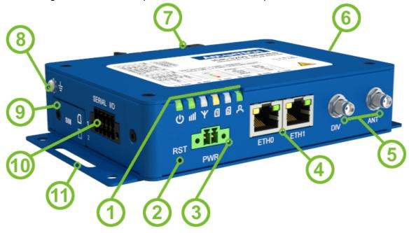
Figure 5: Hardware Overview of the Router
