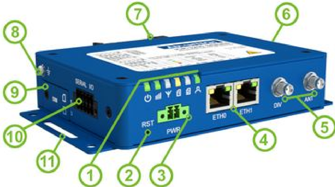
Figure 1: Hardware Overview of the Router
