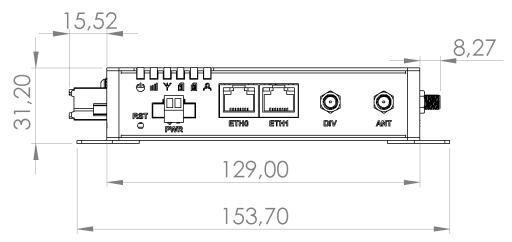
Figure 5: Basic dimensions of the router box
