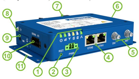
Figure 1: Hardware Overview of the Router
