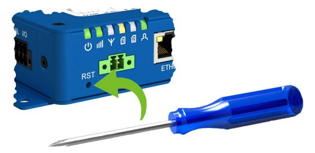
Figure 15: Resetting the Router
