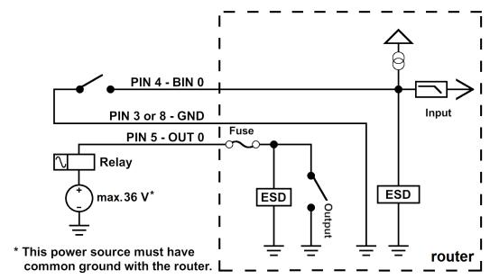
Figure 14: Functional scheme of the binary interface
