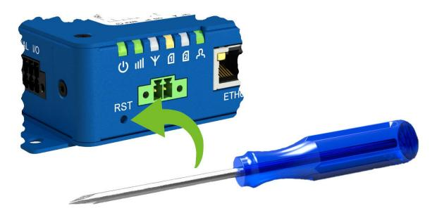
Figure 19: Resetting the Router
