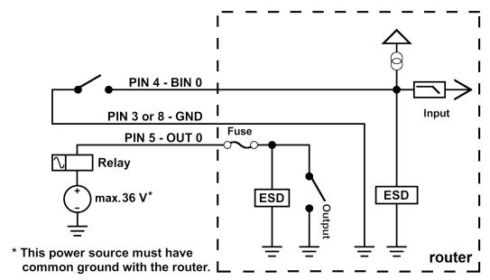
Figure 18: Functional scheme of the binary interface
