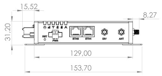
Figure 9: Basic dimensions of the router box
