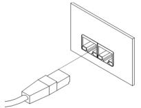
Figure 34: Connection of Ethernet cable
