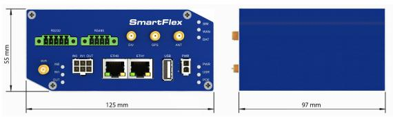
Figure 24: Basic dimensions of the router box
