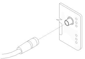
Figure 30: Connecting the antenna
