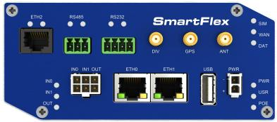
Figure 47: Version with RS232-RS485-ETH interface
