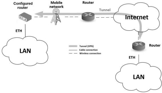
Figure 3: Using VPN tunnel
