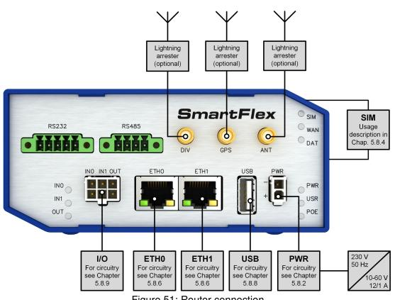
Figure 51: Router connection
