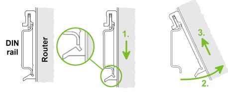
Figure 26: Removal from the DIN rail
