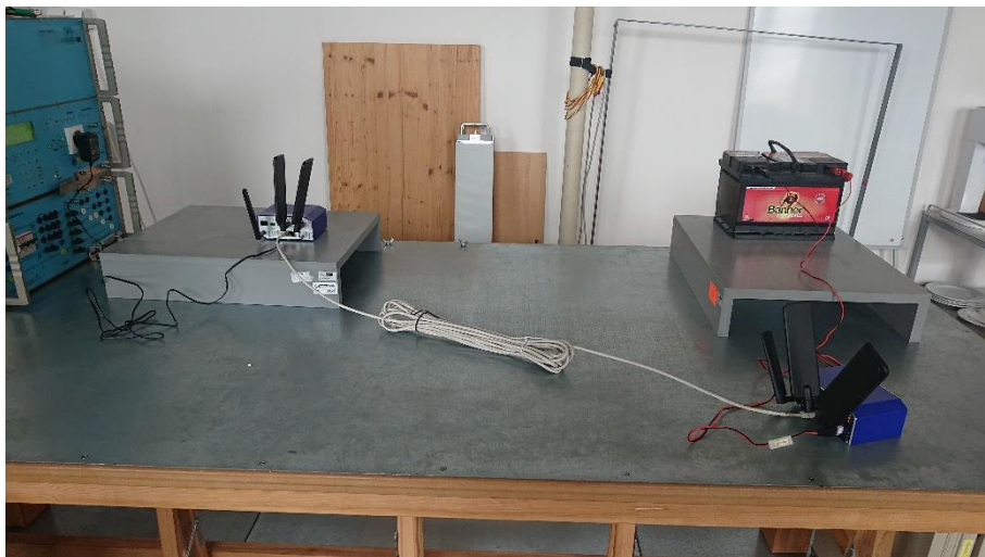
Figure 38: Voltage dips, short interruptions and voltage variations test setup
