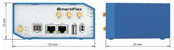
Figure 17: Basic dimensions of the router box
