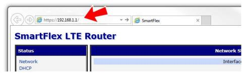
Figure 43: Entering the IP address of the router
