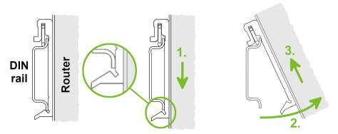
Figure 19: Removal from the DIN rail
