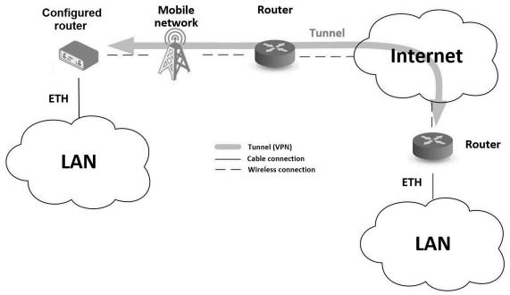
Figure 3: Using VPN tunnel
