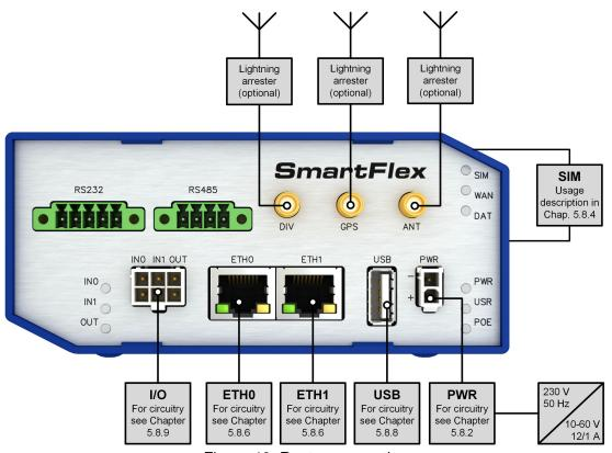
Figure 42: Router connection
