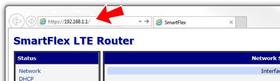
Figure 42: Entering the IP address of the router
