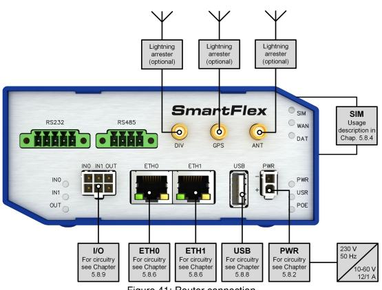
Figure 41: Router connection
