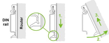
Figure 19: Removal from the DIN rail
