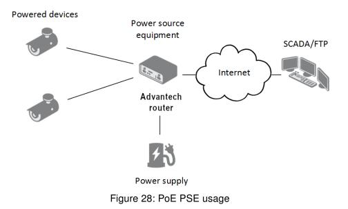
The power supply used with the PoE PSE router has to provide voltage from **44 to 57 V DC** and the output power has to be at least **65 W** for full PoE+ use (Class 4) in both Ethernet ports (ETH0 and ETH1).
