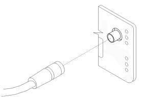
Figure 23: Connecting the antenna
