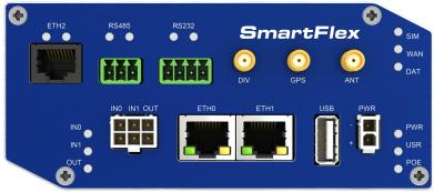
Figure 37: Version with RS232-RS485-ETH interface
