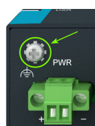
Figure 12: Grounding screw position
